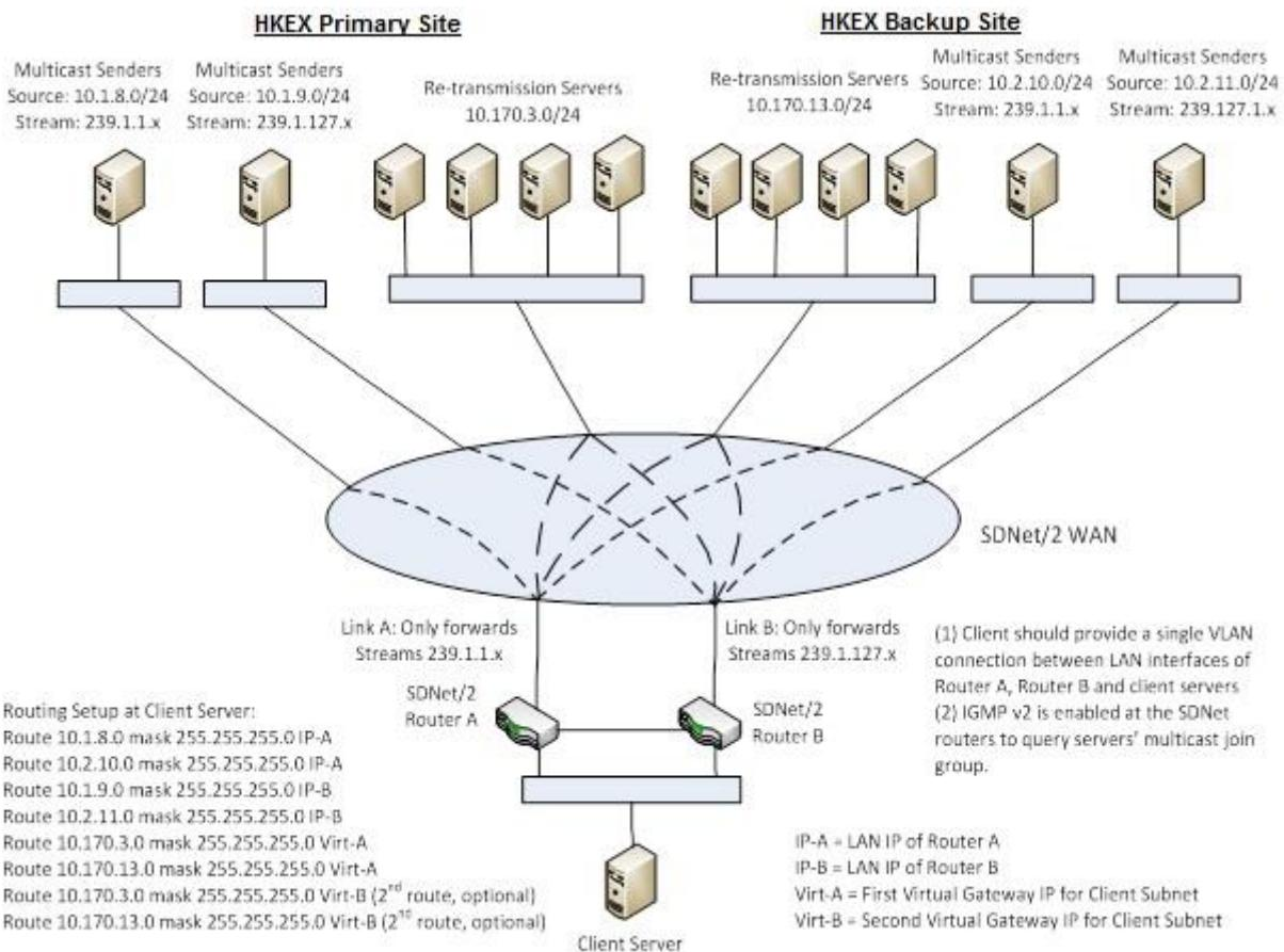
For OMD connection via SDNet/2, a client system has to set up routing to the HKEX host subnets as the diagram depicted. To receive multicast stream, IGMP version 2 is employed at the SDNet/2 routers to query the multicast groups which the client system subscribes. The client system should enable the IGMP function and issue join messages to the SDNet/2 routers for the entitled multicast groups.
