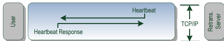
Figure 7: Retransmission Server Heartbeat Message
