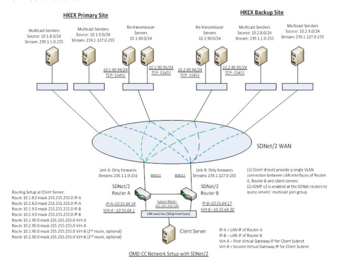
For OMD-CC connection via SDNet/2, a client system has to set up routing to the HKEX host subnets as the diagram depicted. To receive multicast stream, IGMP version 2 is employed at the SDNet/2 routers to query the multicast groups which the client system subscribes. The client system should enable the IGMP function and issue join messages to the SDNet/2 routers for the entitled multicast groups.
