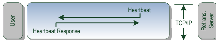
Figure 7: Retransmission Server Heartbeat Message
