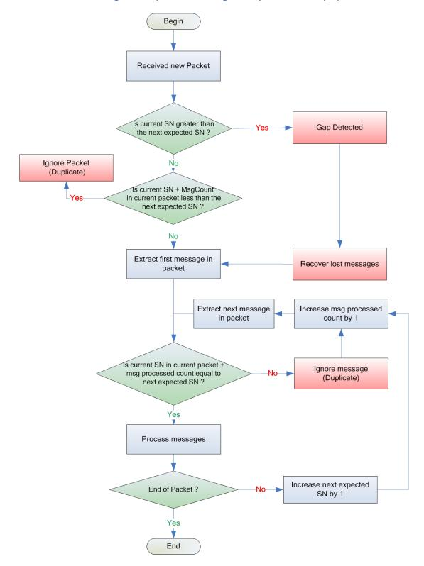
Figure 2: Gap Detection using the Sequence Number (SN)
