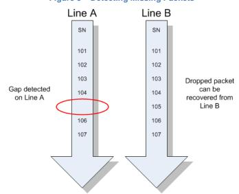
Figure 3 – Detecting Missing Packets
