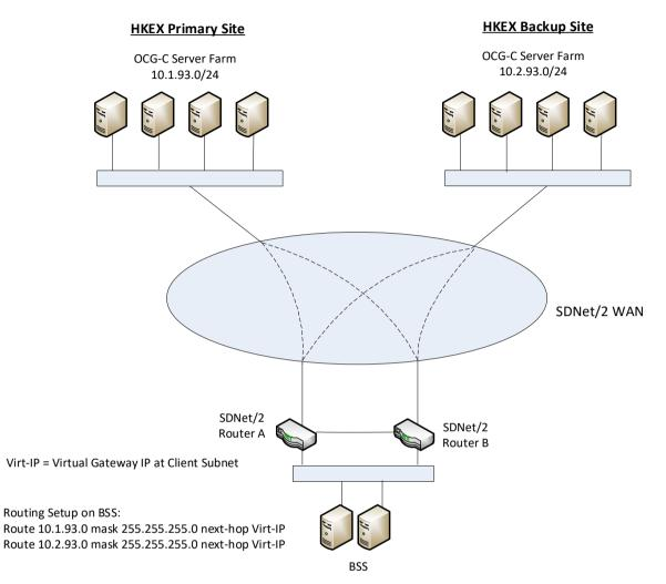
Figure-2 BSS Network Setup for OCG-C
