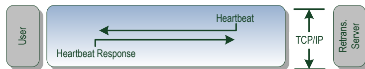
Figure 7: Retransmission Server Heartbeat Message
