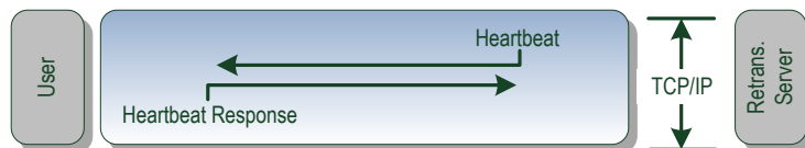
Figure 7: Retransmission Server Heartbeat Message
